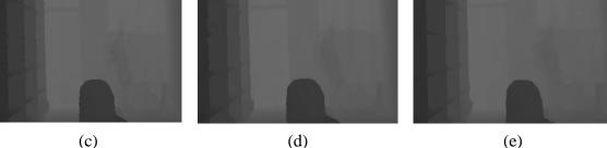
Fig. 6 (a) is color image, (b) is raw depth image, (c) is inpainted by (Qi et al., 2013), (d) is inpainted by (Camplani and Salgedo, 2012), (e) is proposed method
